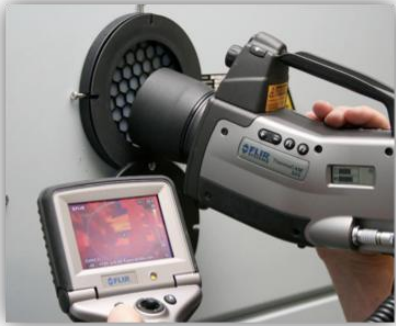
Figure 1a (left) shows an IRISS infrared window installed in electrical cabinet 2 . The thermographer holds an IR camera against an IR window to see inside the switchgear. These windows can be custom fit to any data center equipment.
