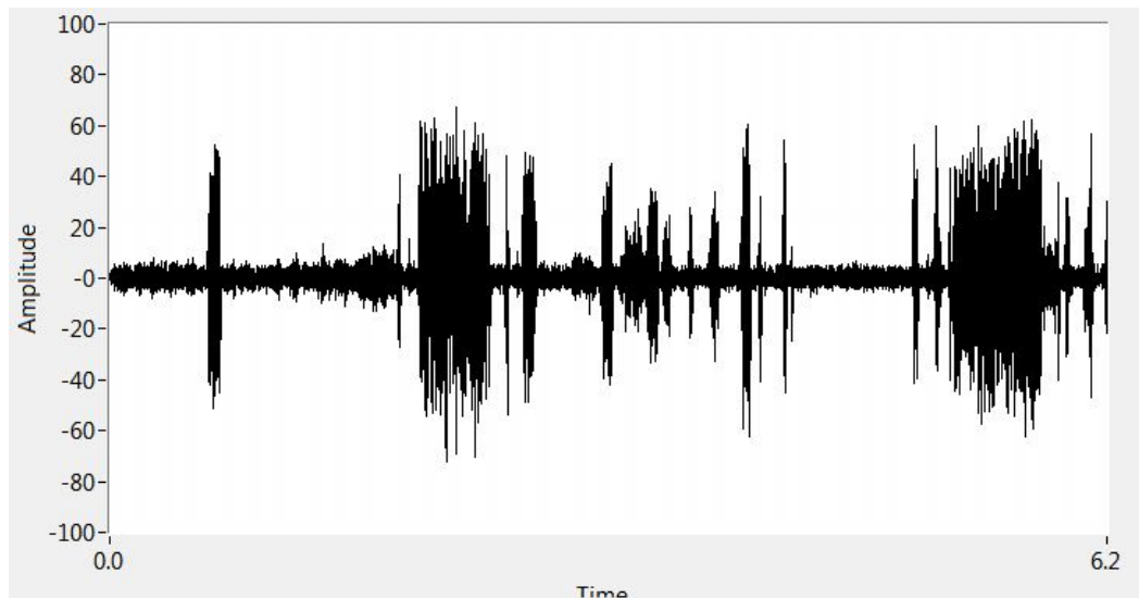
Arcing as seen in the Time Wave Form. Notice the lack of uniform harmonics and the sudden starts and stops of the discharge
