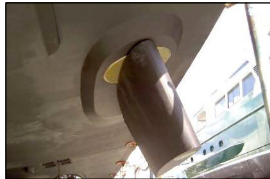
Lead portion of the stabilizer systems mounting and backing installation looking aft after the reconstruction and repairs.
