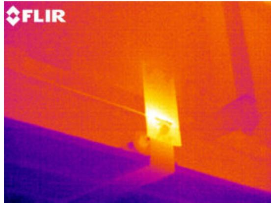
The images below are of a bad conveyor bearings. The only way to find these before failure is with infrared. There are 79 miles of conveyor with a bearing set every 8 to 10 feet. You do the math. OK, I will - let's see, carry the 2...that's over 40,000 pairs of bearings!
