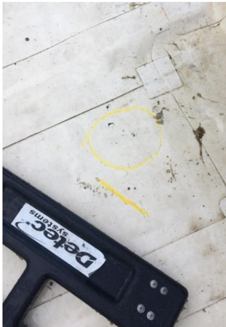
Figure 8: Breach found in a conventional roofing assembly with conductive primer under the membrane.
