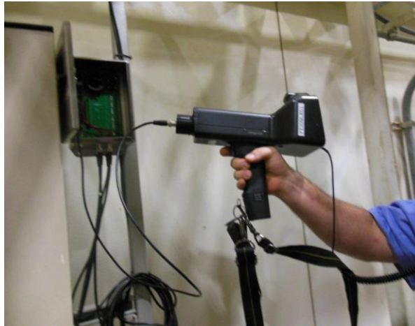
The above image shows an ultrasound instrument connected to a four channel switch box.
