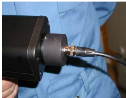
A remote access sensor with cable mounted to the outboard bearings on a motor (left). The other end of the RAS cable connected directly to a portable hand-held ultrasound instrument (right).
