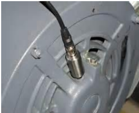
A remote access sensor with cable mounted to the outboard bearings on a motor (left). The other end of the RAS cable connected directly to a portable hand-held ultrasound instrument (right).
