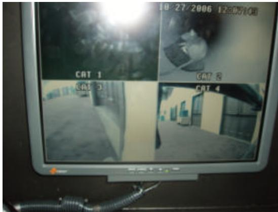
**Typical quad screen of a surveillance system**
