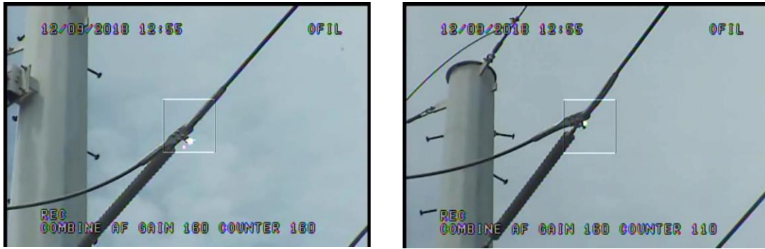
Figure 9: shows examples of corona detected on cotter pin connections at the live end of the end-end inspector.
