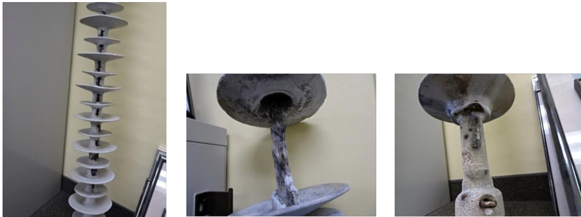
Figure 1: Showing rupture pattern on polymer insulator; dark areas between sheds in the failure pathway the fault followed to ground. Middle photo shows sheds closer to live end and photo on left is the ground side; show existing path of electrical fault.
