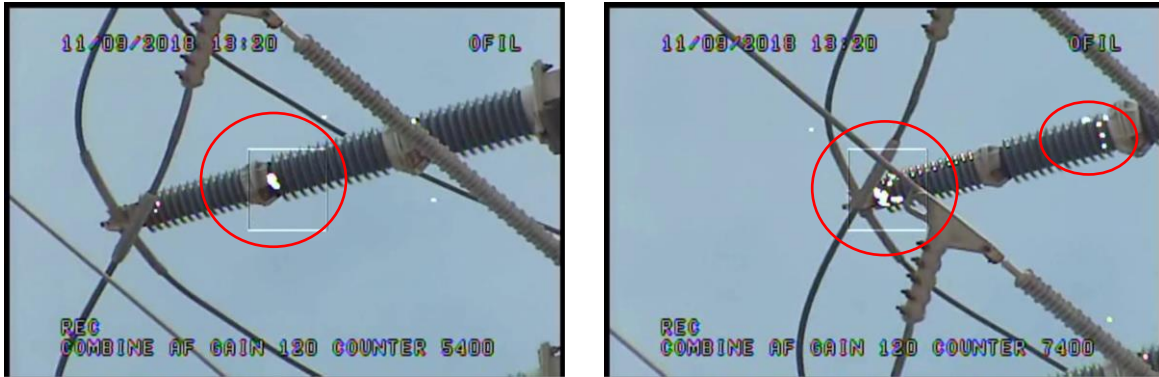
Figure 7: shows examples of corona detected on ceramic stand-off insulators at the bolted joint and the live-end mechanical shoe attachment
