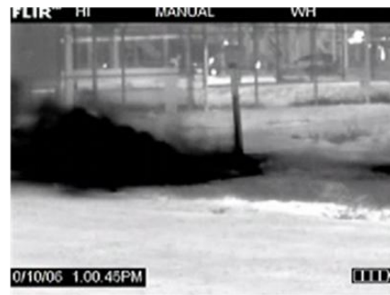
CH4 Pipeline Ground Leak
