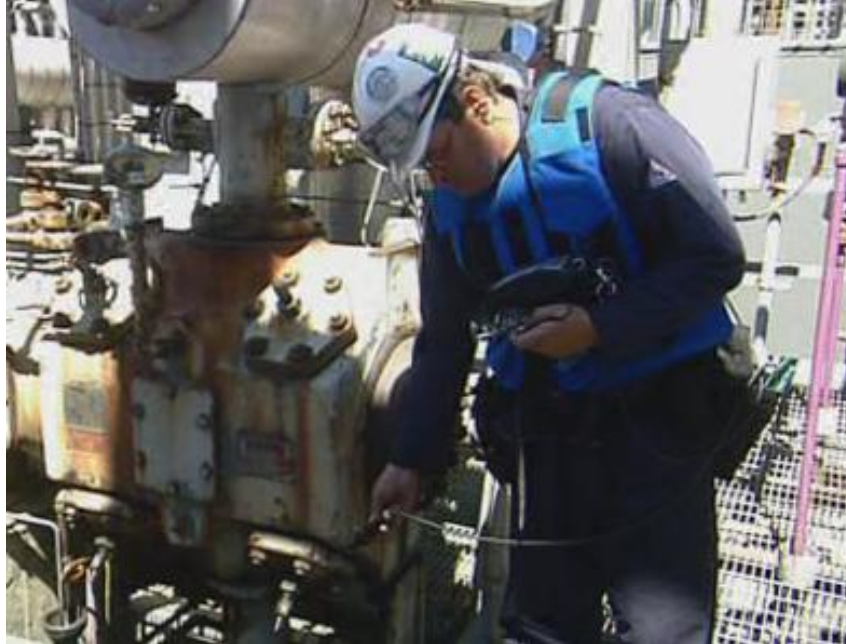
Figure 2. Toxic vapor analyzers (also called “sniffers”) are labor intensive, but can quantify the leak rate
