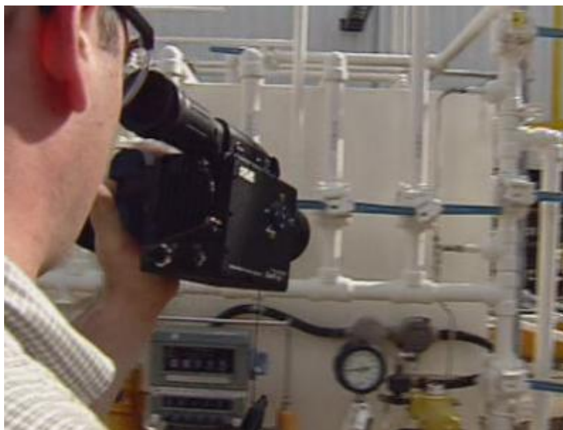
Figure 3. Typical usage of an IR camera for VOC leak detection
